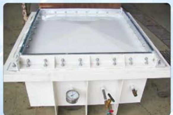
Test for Hydraulic Pressure
