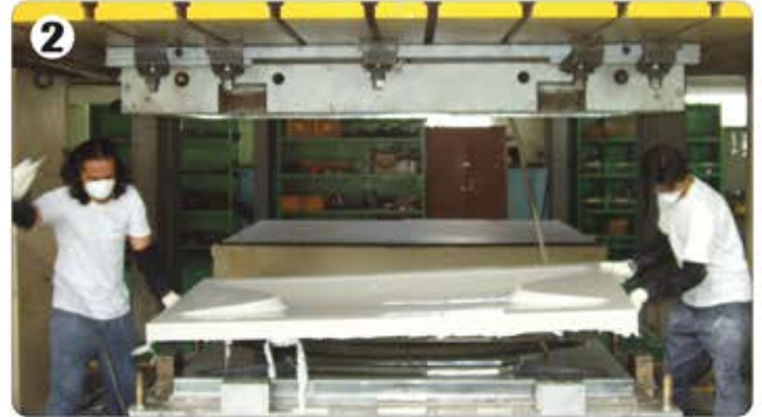
Molded by hot hydraulic press
